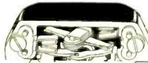
Arrangement of the commutator parts and spring-arm of the new Hubbell snap switch described at the left.
